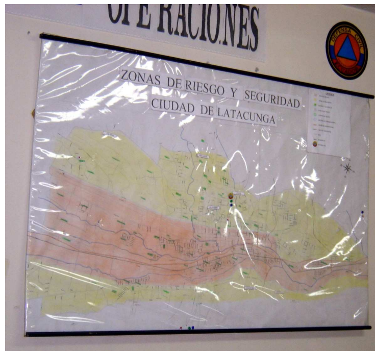
Figure 4 Civil Defence lahar hazard map of Latacunga, showing the high and moderate lahar danger zones (orange and yellow, respectively) over the street layout; much of the city is at risk.
