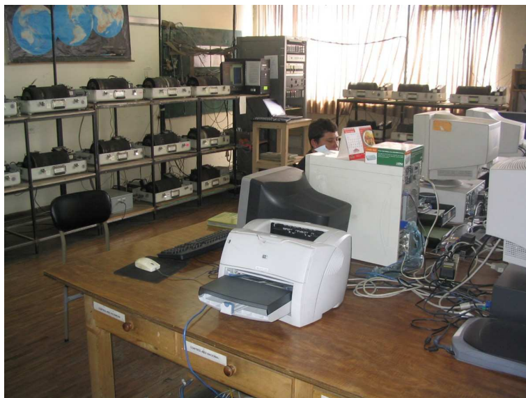
Figure 6 Computer and smoker-drum monitoring and recording of radio-telemetered seismograph data at Instituto Geofísico in Quito. Earthquake locations are calculated here and Civil Defence is alerted to those indicating eruptions. Staff and students are rostered to provide a constant monitoring presence.
