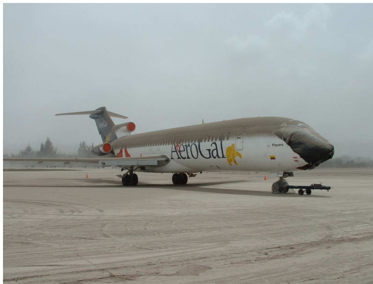
Figure 10 Average jet airliners were able to be cleaned by high-pressure water blasting from standard fire appliances in 10 to 15 minutes. No water ingress was detected, and no leachate or abrasion damage was noted. Aircraft maintenance experts were on hand to monitor effects. Note the covering of engines and nose cone prior to ash fall.
